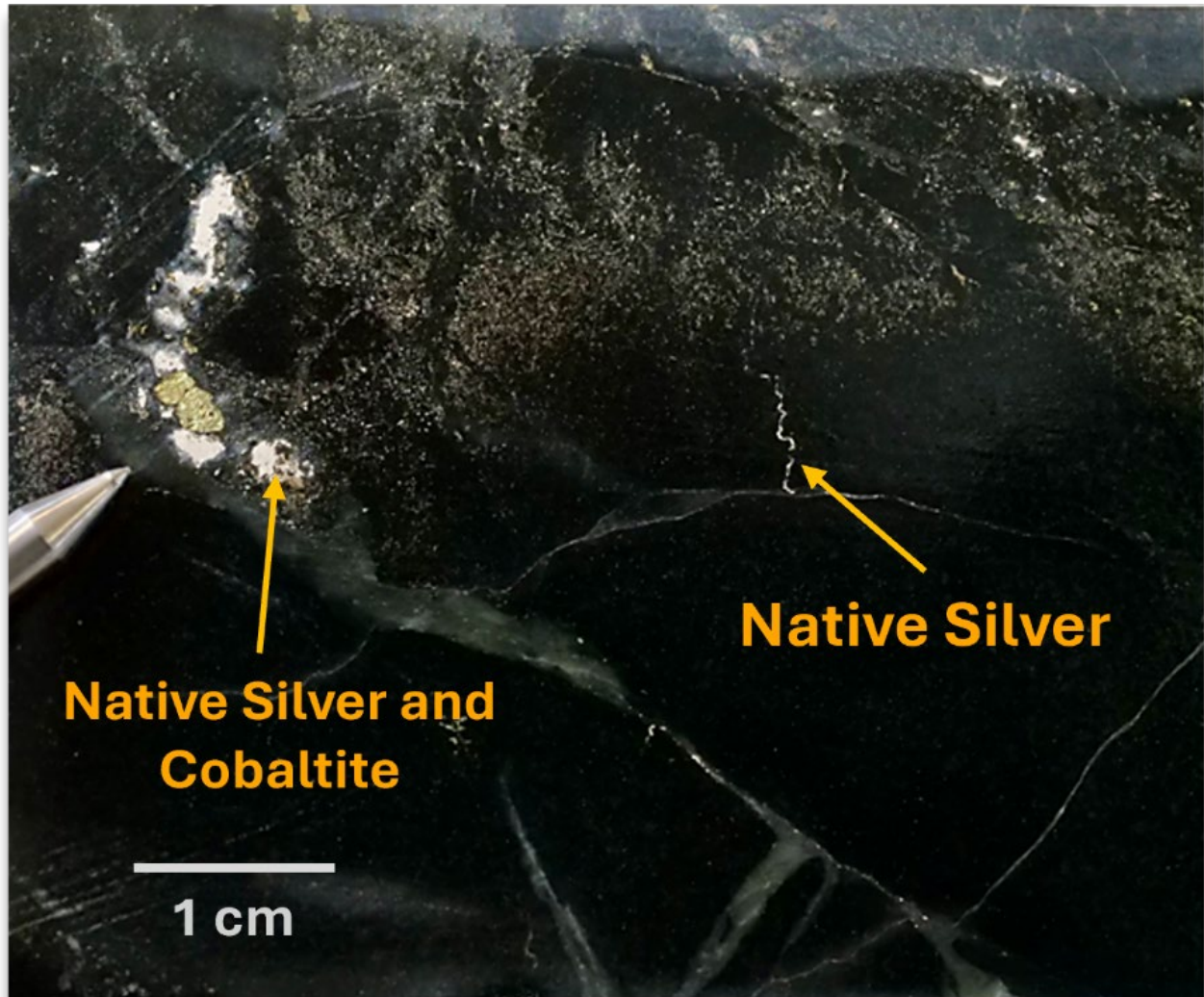
Figure 2. Detailed NQ core photograph of hole LM-26-341 at 108.7 m showing native silver only and native silver + cobaltite in carbonate + sulphide veins.
