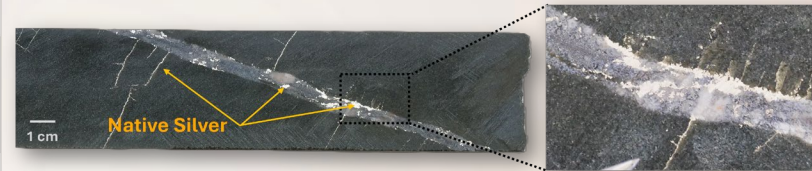
LM-26-350 at 115.25m, displaying native silver (appearing white) as veinlets and blebs.
