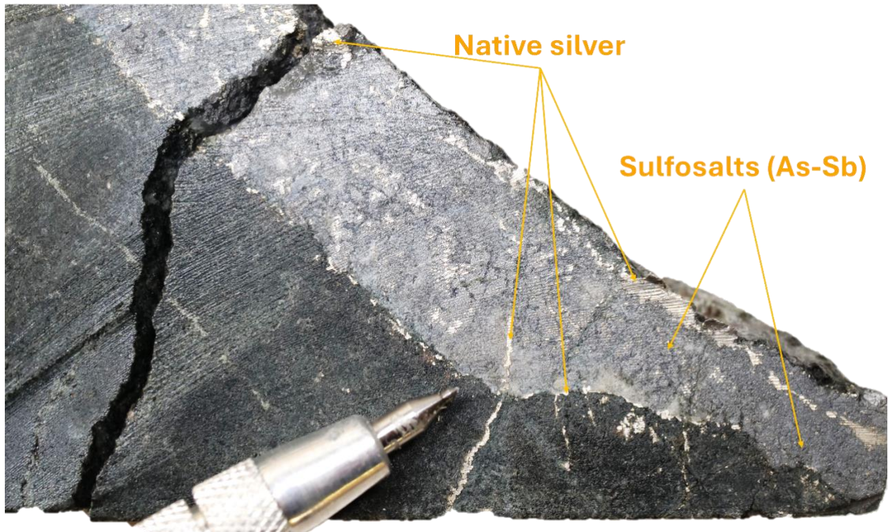
Figure 6. Photograph of NQ Core LM-26-301 at 115.65m, of native silver within carbonate veins.
