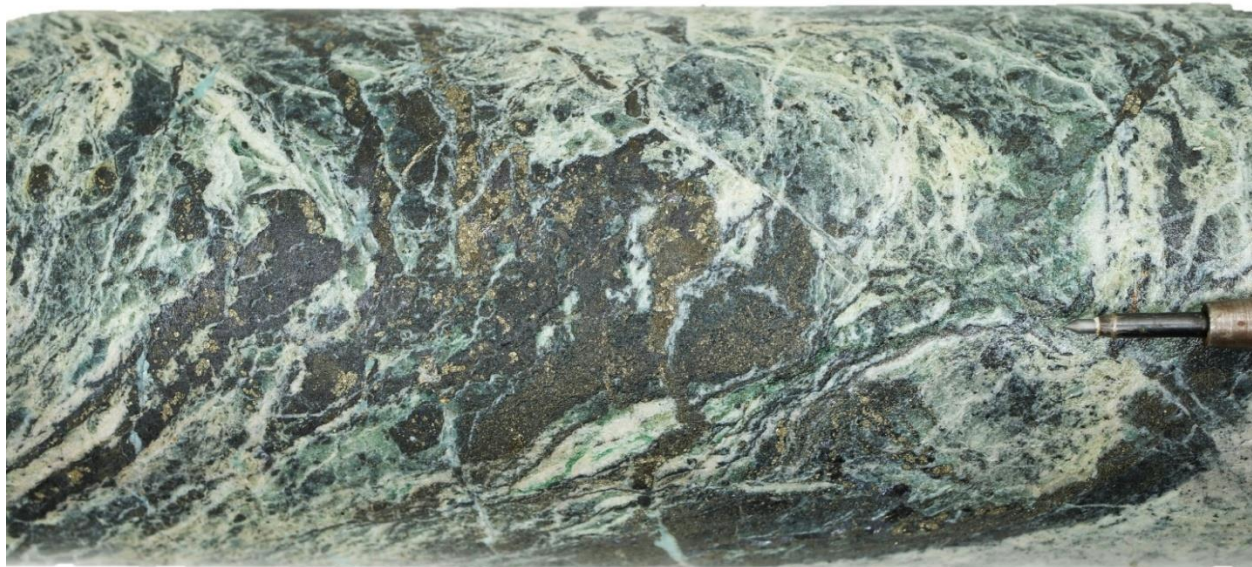
Figure 4. HQ drill core photograph of hole THN25-364 at 152 meters showing pyrite-sphalerite-galena-chalcopryrite vein hosted in sericite-chlorite-calcite altered Stuhini volcanoclastics.
