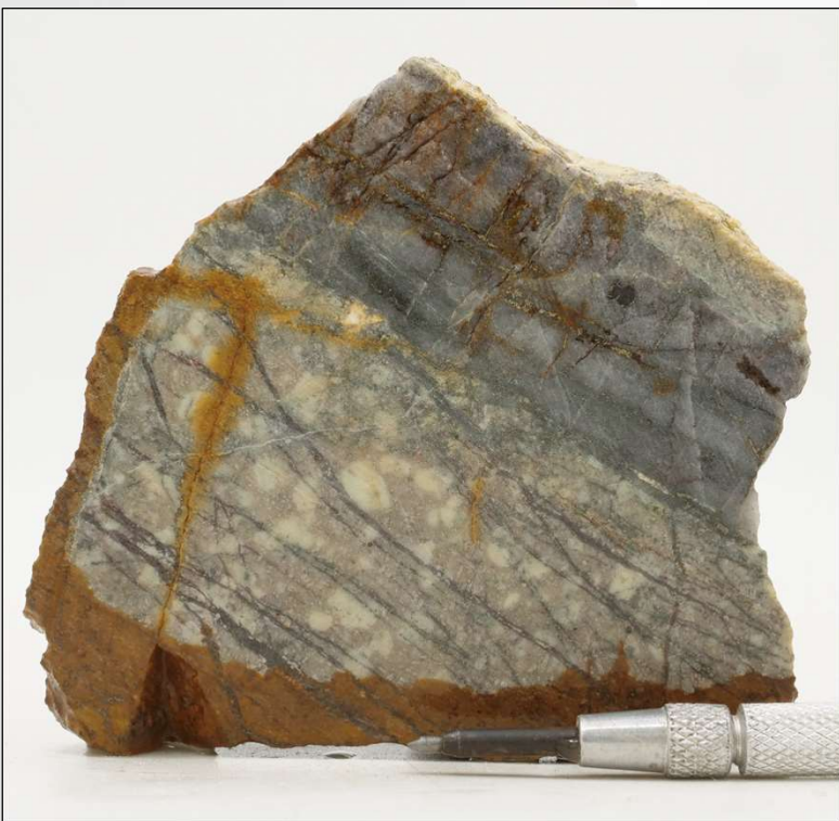
D201227 - quartz-chalcopyrite-molybdenite A veins - 0.51% Cu, 1.11 g/t Au, 36 ppm Mo
