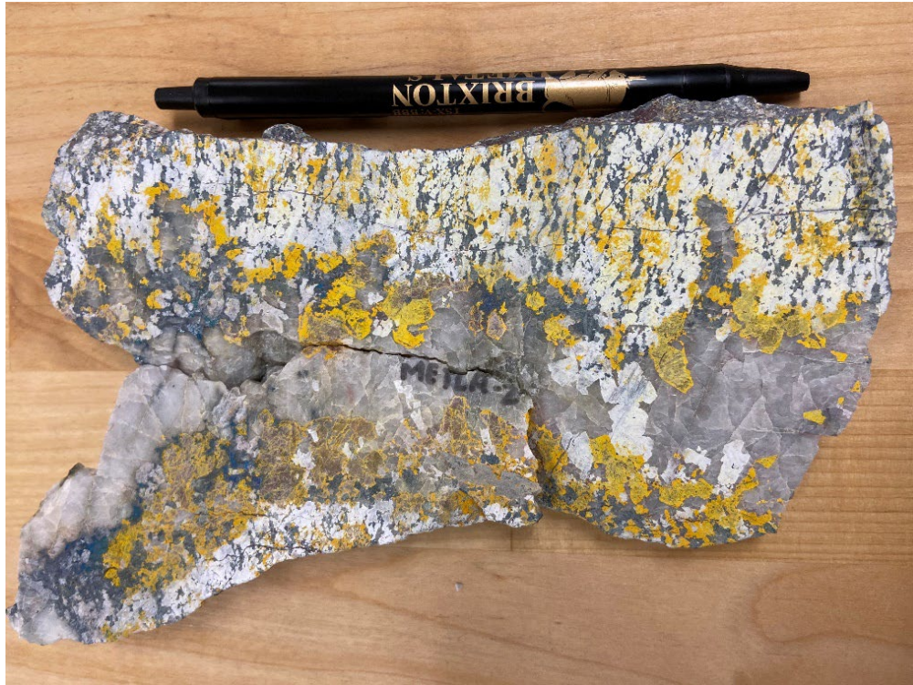
Figure 3. Stuhini Rock Float Sample ALW19-004 of Foliated Diorite Porphyry with Bornite-Chalcocite returning 4.7% Cu, 1.8 g/t Au, 31 g/t Ag, 0.3 g/t Pd (after HF Acid Staining, Potassic Alteration in Yellow).
