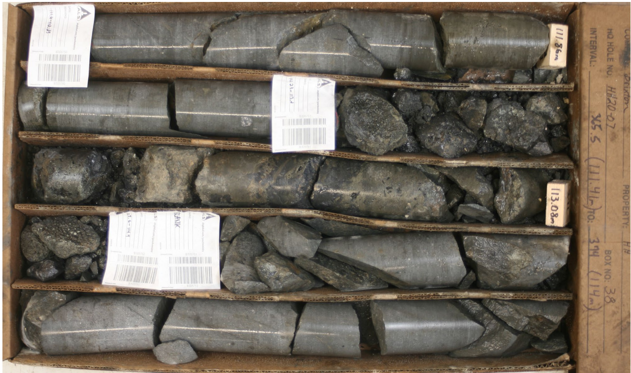
Figure 4. HQ Core from Hole HH20-07: Massive Sulphide from 112.23 – 113.20m depth (0.97m of 1,885 g/t Ag, 4.68 g/t Au, 15.20% Cu). Box includes 111.41-114.00m.
