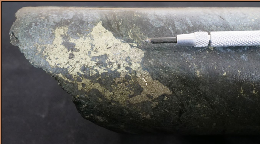
THN22-231 at 793.85m: 1.50m of 0.42g/t Au, 12.1 g/t Ag, 0.77% Cu & 152.50ppm Mo Mt-Py-Cpy D-Vein hosted in SLTS
