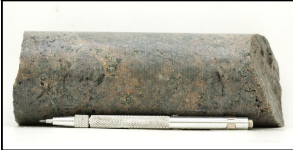
THN24-312 at 360.68m - quartz-pyrite-chalcopyrite-magnetite veins with potassium feldspar alteration halo
