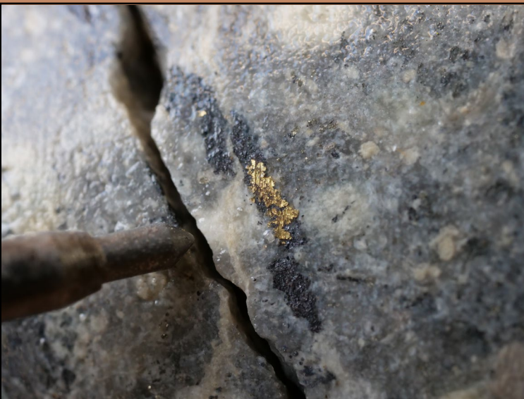
THN22-237 at 159.78m: 0.38m of 34.5 g/t Au Visible Gold hosted in Quartz Diorite
