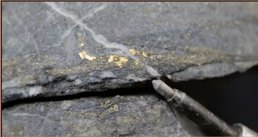
THN22-25 at 151.75m: 0.25m of 249 g/t Au Native Gold hosted in Quartz Diorite
