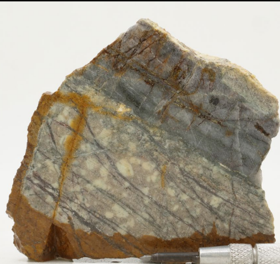
D201227 - quartz-chalcopyrite-molybdenite A veins - 0.51% Cu, 1.11 g/t Au, 36 ppm Mo
