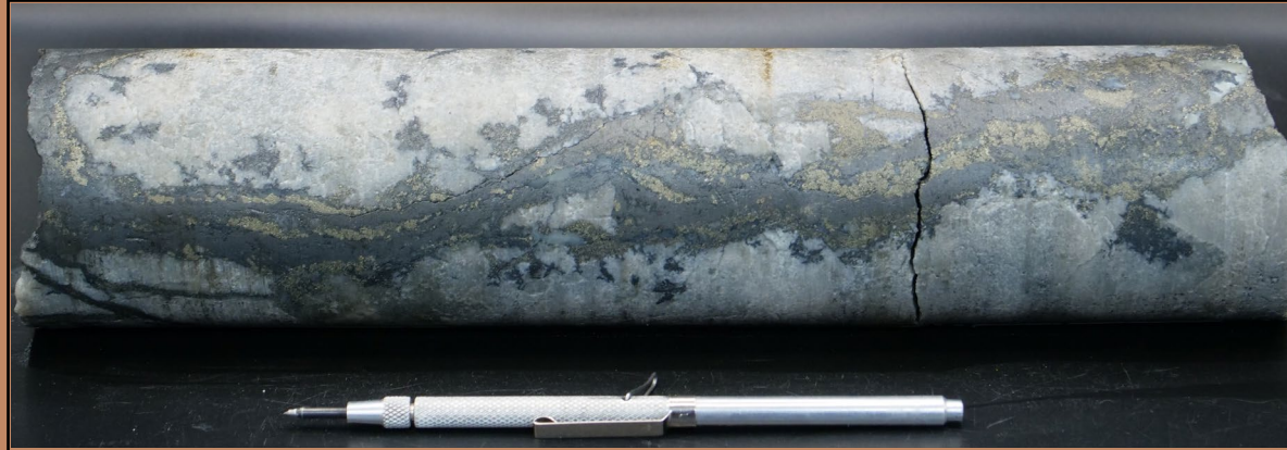
172.60m: 1.50m of 0.63g/t Au, 159.0g/t Ag & 2.74% Cu Py-Ss Vein hosted in Porphyry Y
