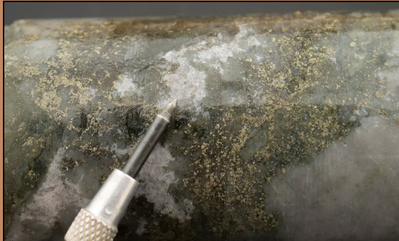
THN22-221 at 1040.25m: 2.00m of 0.20g/t Au, 5.13g/t Ag, 0.69% Cu & 254ppm Mo Mo-Cp Vein hosted in Porphyry X
