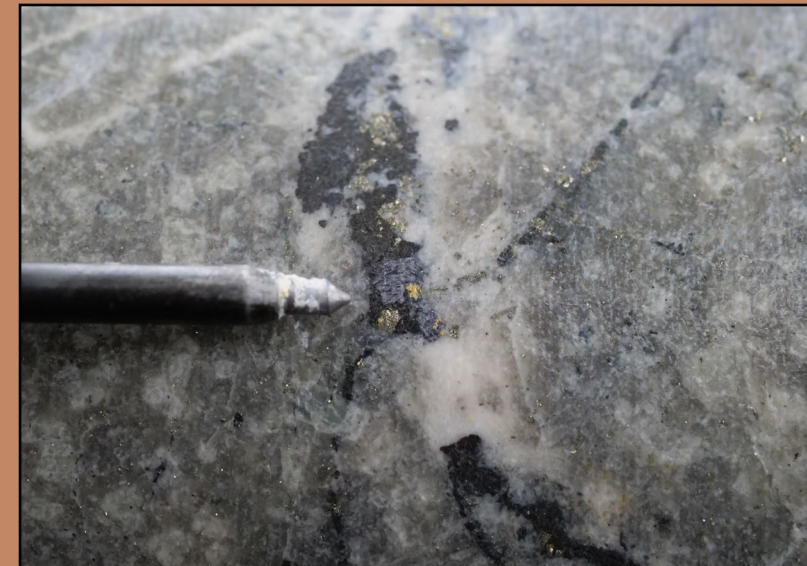
THN22-208 at 23.51m: 0.25m of 40.60 g/t Au Visible Gold hosted in a base metal vein
