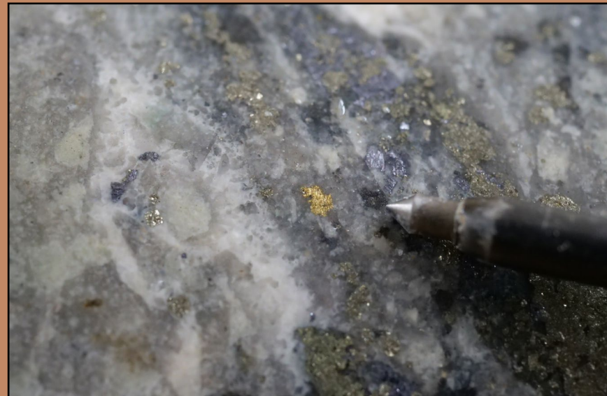
THN22-255 at 61.77m: 0.30m of 15.45 g/t Au Visible Gold hosted in Quartz Diorite
