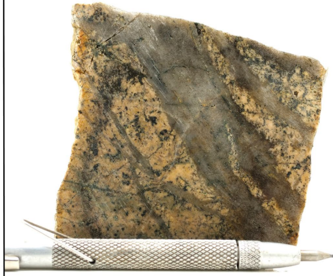
Porphyry style stockwork quartz veins commonly found at Sentinel within muscovite-phengite-specularite altered felsic volcanics
