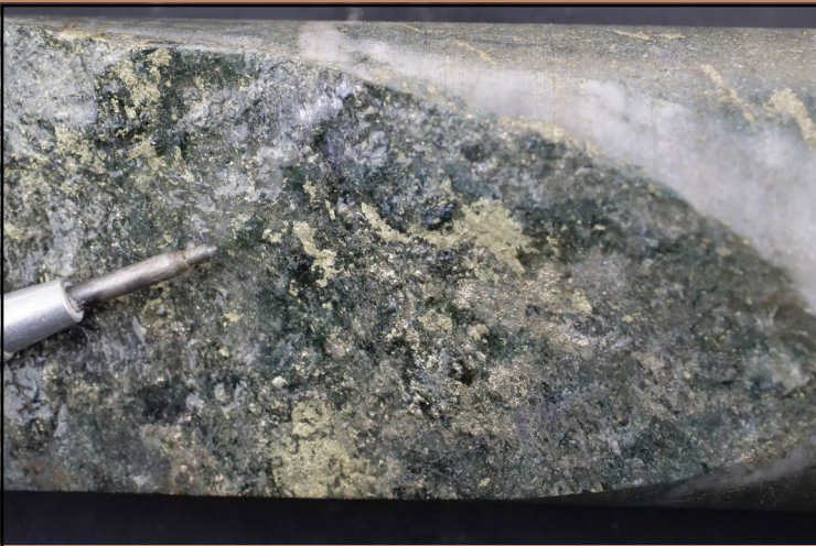
THN22-201 at 1023.10m: 1.9m of 0.60g/t Au, 8.81g/t Ag, 1.14% Cu & 250ppm Mo Cpy on fractured surface hosted in SLTS
