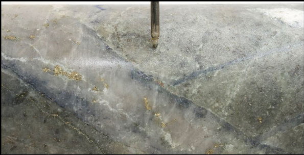
THN24-312 at 431.00m - quartz-molybdenite-pyrite vein in QSP altered diorite porphyry
