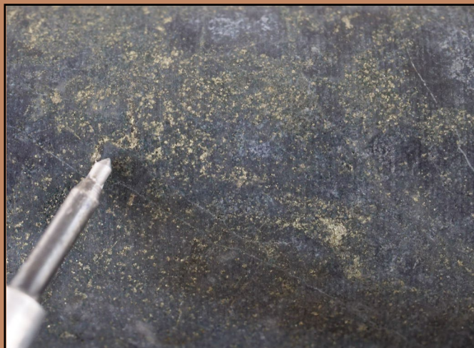
THN22-201 at 1112.89m: 2.00m of 0.40g/t Au, 7.80g/t Ag, 1.10% Cu, 591ppm Mo Disseminated Py-Cpy hosted in SLTS
