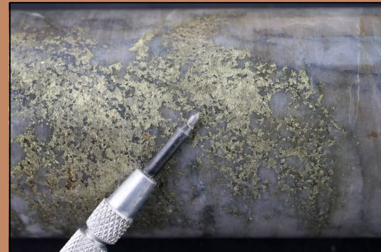
THN22-201 at 1092.90m: 2.00m of 0.14g/t Au, 9.30g/t Ag, 0.78% Cu & 395ppm Mo Py-Cpy D-vein hosted in Porphyry X
