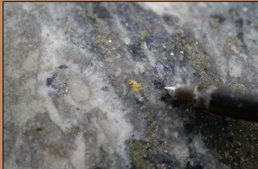
THN22-255 at 61.77m: 0.30m of 15.45 g/t Au Visible Gold hosted in Quartz Diorite
