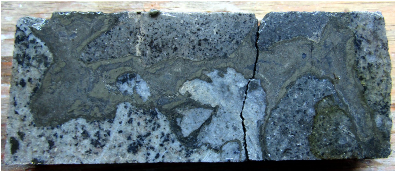
Figure 3. THN19-151 HQ core from 142.19m depth, matrix filled pyrite-sulphosalts-sphalerite.
