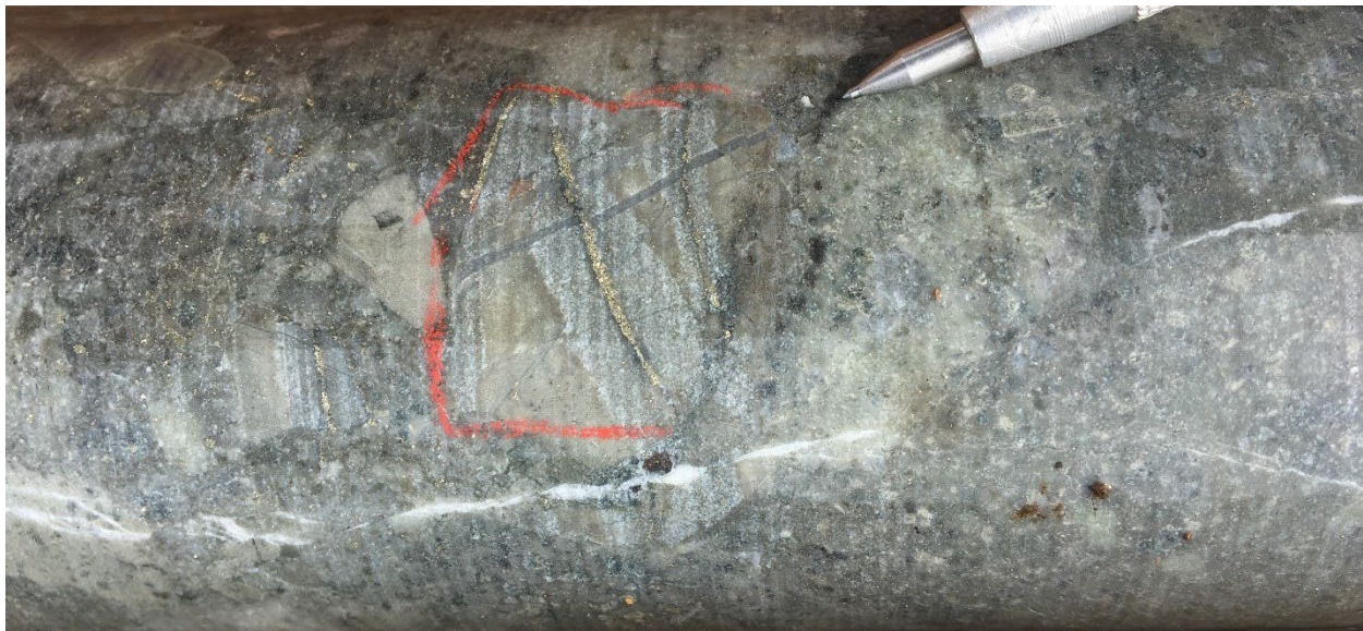
Figure 8. THN19-150 core from 442.30m porphyry clast with pyrite-quartz-chalcopyrite.
