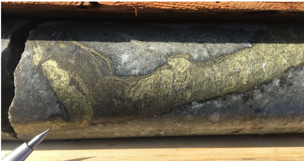
Figure 5. THN19-150 core from 296.50m depth, matrix filled chalcopyrite-sulphosalts-pyrite.
