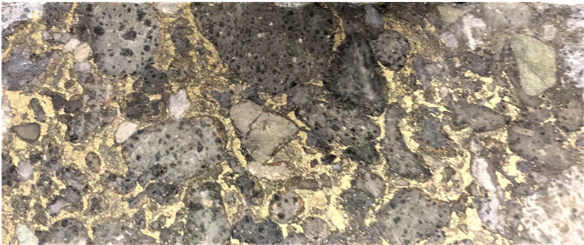
Figure 7. THN19-150 of close up of core from 421.12m depth (~4% Copper), matrix filled chalcopyrite.
