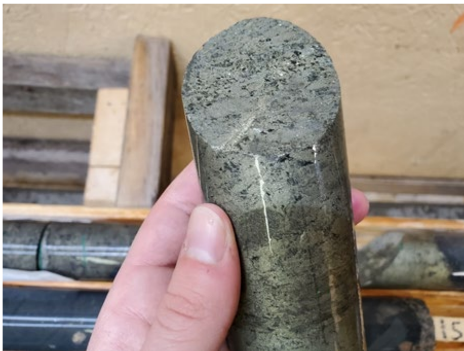
Figure 4. Hole LM-20-111 at 113.0m to 113.5m, Massive Chalcopyrite, Pyrite, and Pyrrhotite Hosted within Conglomerate, returned 10.85% Cu, 39.6 g/t Ag, 0.05% Co over 0.5m.
