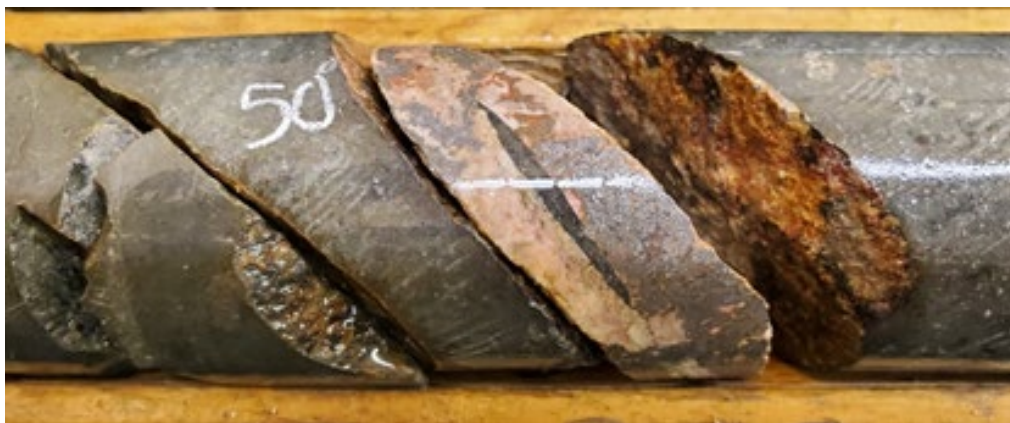
Figure 3. Hole LM-20-113 from 5.9m, Native Silver and Cobaltite in Quartz-Carbonate Veins.
