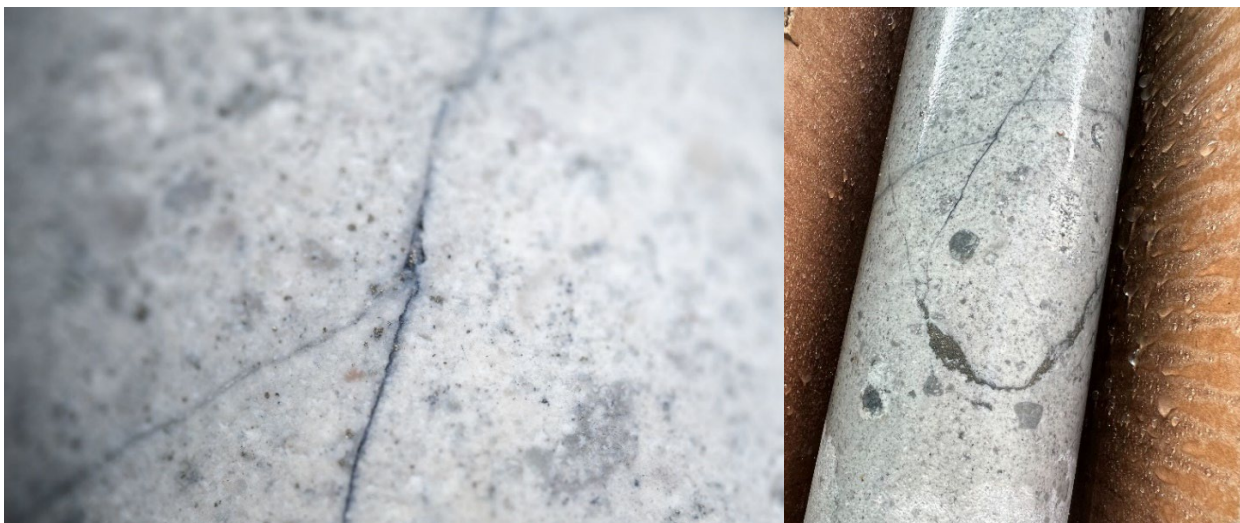
Figure 3. Photo of fine early quartz veins with clear alteration halos cut by later molybdenite-pyrite veins observed in drill core from HHD-004 at 1241.9 meters depth. Molybdenite veins such as this are commonly observed in the outer portions of mineralized porphyry systems.
