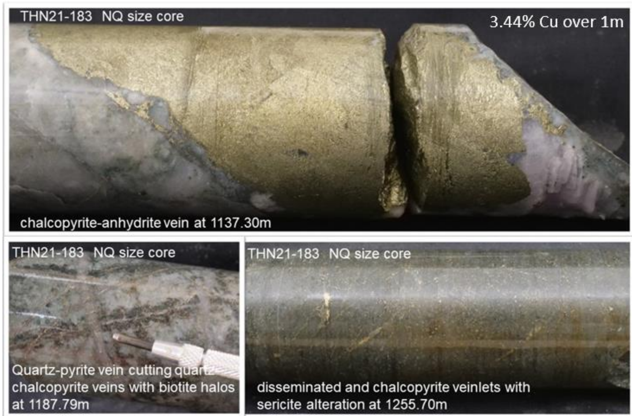
Figure 7. Drill Core at 1137.3m, 1187.79m and 1255.70m Depth.
