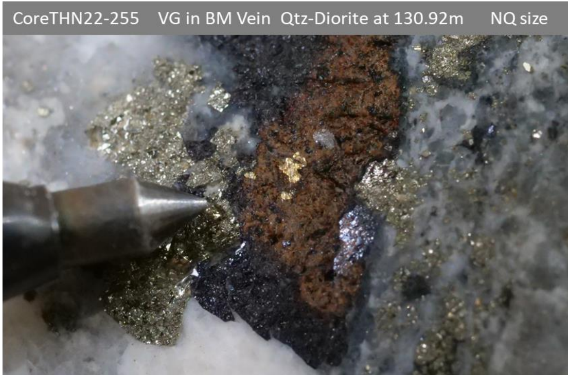
Figure 4. Visible Gold Photograph of HQ Core from Hole THN22-255 at 130.92m Depth.
