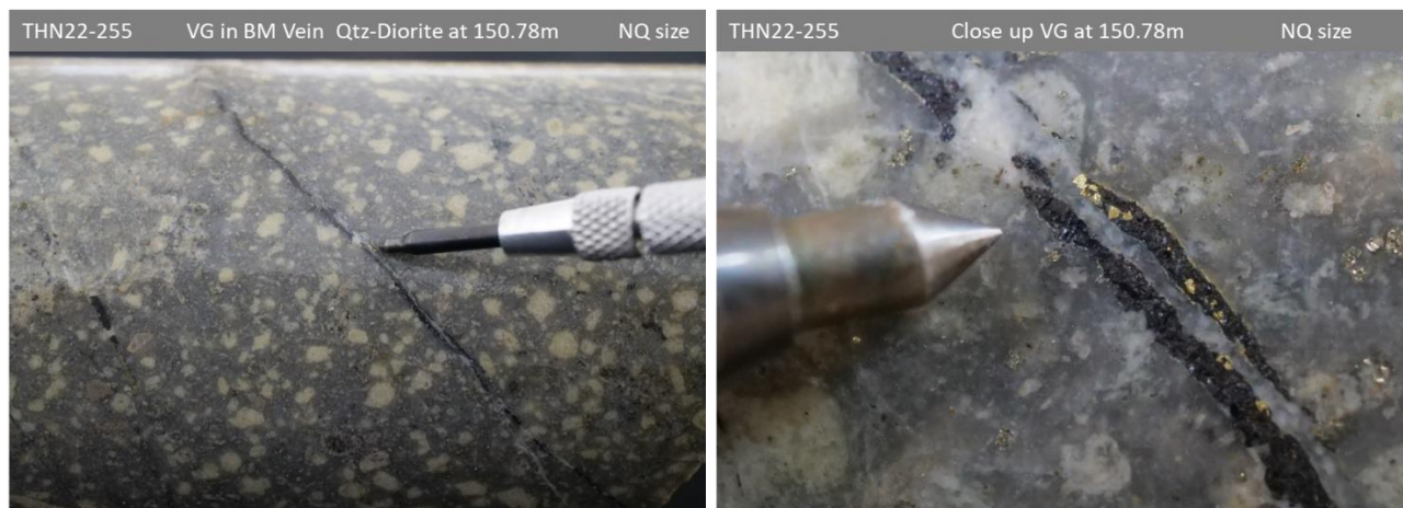
Figure 5. Visible Gold Photographs of HQ Core from Hole THN22-255 at 150.78m Depth.
