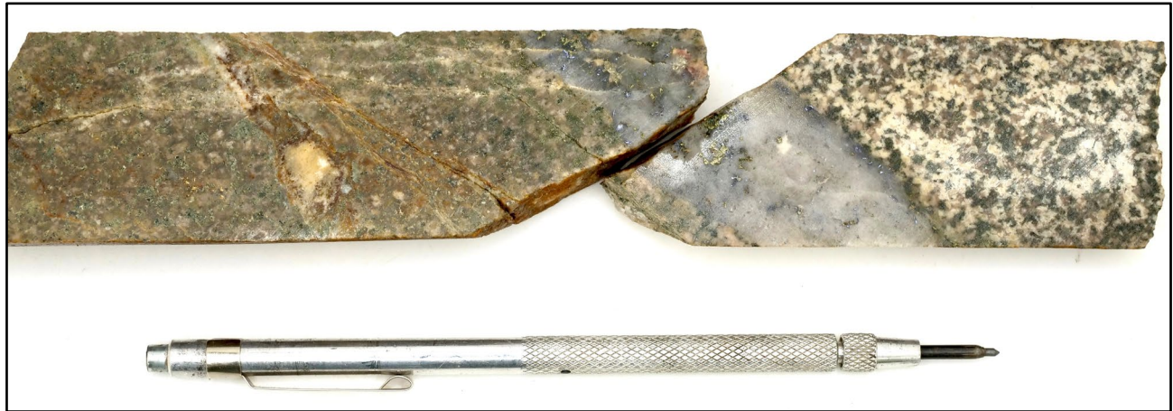
Figure 3. BQ sized core from Julian Mining's 1965 Cirque Program. Select unanalyzed core containing chalcopyrite and molybdenite in quartz vein.
