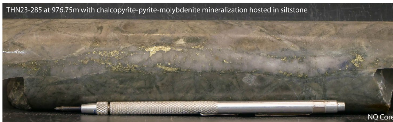
Figure 2: Hole THN23-285 Core Photograph at 976.75m Depth from a 1.00m Interval that Assayed 0.35% Cu, 207 ppm Mo.
