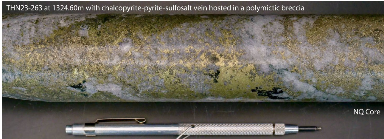
Figure 6. Hole THN23-263 Photograph of Mineralized Core at 1324.60m Depth from a 1.00m Interval that Assayed 2.64% Cu, 473 ppm Mo, 34.7 g/t Ag, 0.27 g/t Au.
