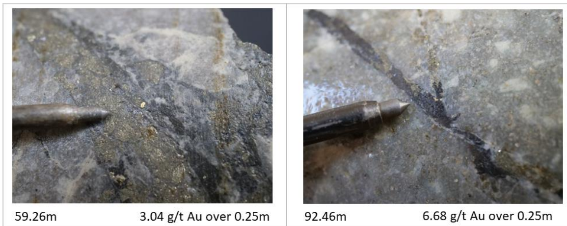
Figure 7. Visible Gold Photographs of HQ core from hole THN22-248.
