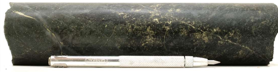
NQ Core at 1372.00m: Chalcopyrite-pyrite veining and disseminations hosted in Hornfels Siltstone
