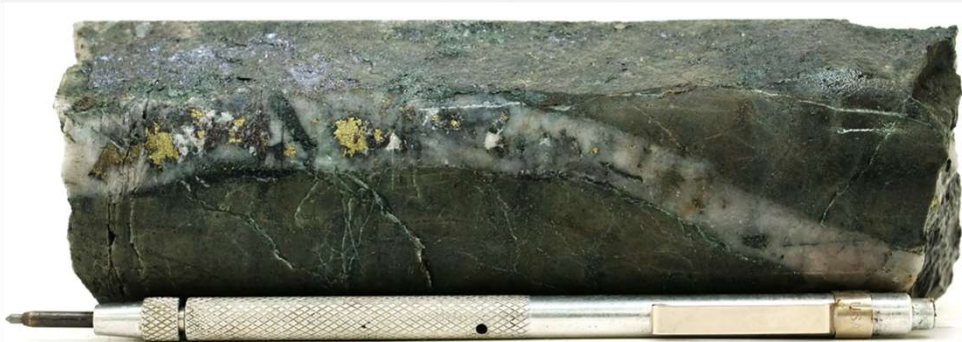
NQ Core at 1372.00m: Chalcopyrite-pyrite veining and disseminations hosted in Hornfels Siltstone
