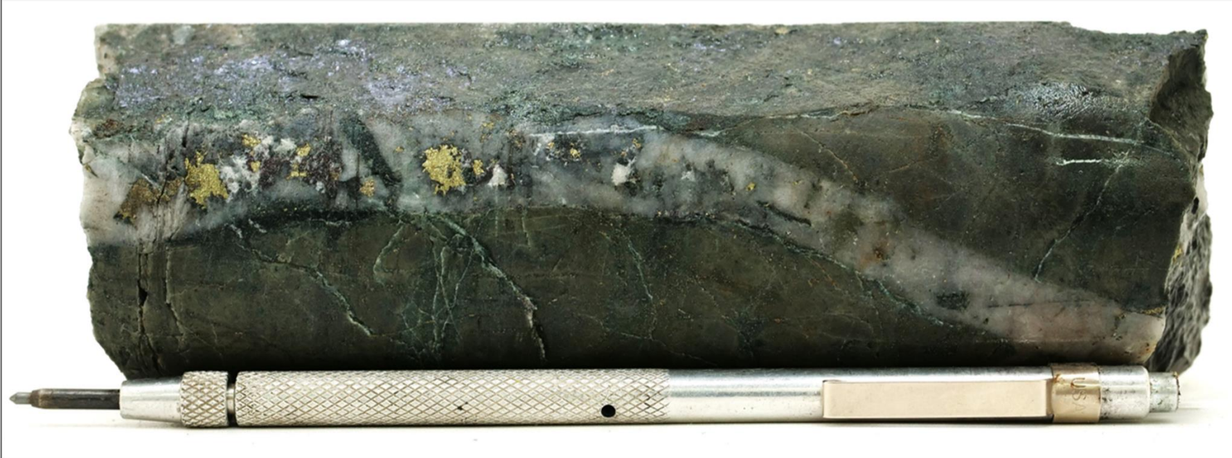
NQ Core at 1372.00m: Chalcopyrite-pyrite veining and disseminations hosted in Hornfels Siltstone
