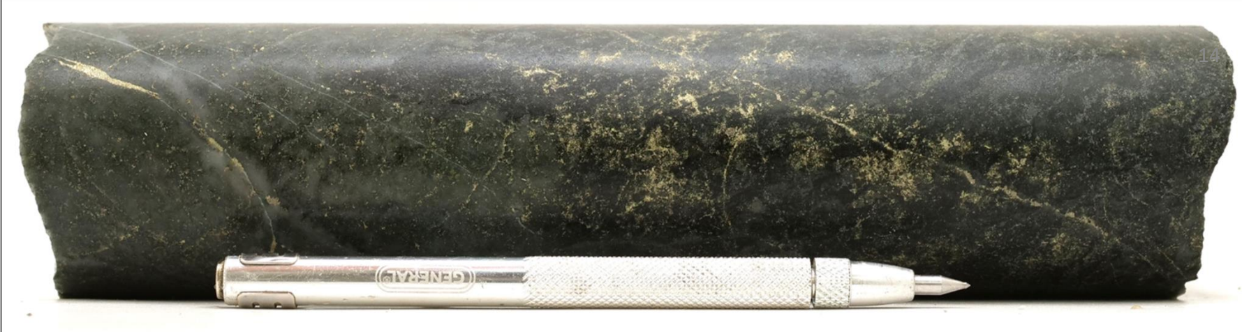
NQ Core at 1372.00m: Chalcopyrite-pyrite veining and disseminations hosted in Hornfels Siltstone
