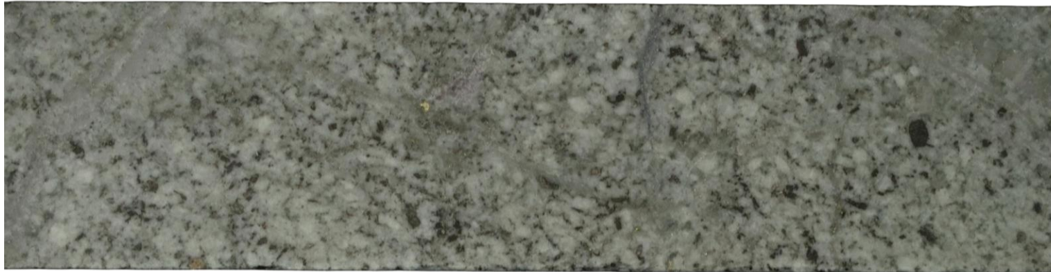
Porphyry X – Crowded Feldspar Porphyry with Stacked Biotite THN23-261 NQ Size Core at 1448.65m
