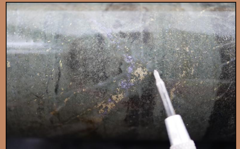
THN22-213 at 938.85m: 1.00m of 0.39g/t Au, 5.42g/t Ag, 0.85% Cu & 187.5ppm Mo Py-Mo hosted in Mineralized Mafic Dyke
