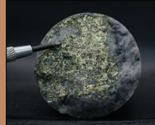
1461.85m: 2.00m of 0.64% Cu & 1215ppm Mo Cpy A-vein hosted in Porphyry X
