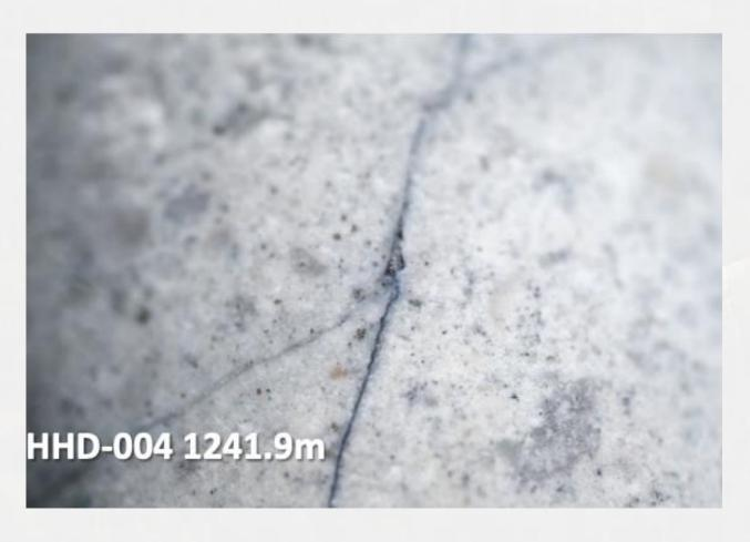
Fine early quartz veins with clear alteration halos cut by later molybdenite-pyrite veins. Molybdenite veins such as this are commonly observed in the outer portions of mineralized porphyry systems.
