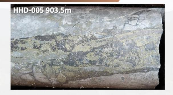
Sub-vertical pyrite-enargite vein cutting diatreme breccia. The presence of gold- and copper-rich veins at depth in HHD-005 are indicative of a vertically extensive hydrothermal system and suggests proximity to a high-grade feeder zone.
